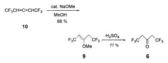
with  $H_2SO_4$  for 2 h at 100 °C. In contrast, methanol added across the C=C double bond under mild conditions (10–20 °C) in the presence of a catalytic amount of NaOCH<sub>3</sub> to give the methyl vinyl ether **9** in 88% yield. The latter hydrolyzed readily (H<sub>2</sub>SO<sub>4</sub>, 15–20 °C, 0.5 h) to give ketone **6** (77% yield).
